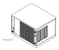
3) Clean the condenser using a vacuum cleaner, soft brush, or low-pressure air. Clean from bottom to top, not side to side. Be careful not to bend the fins of the condenser.
