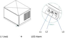
L1 (red) → LED Alarm L2 (orange) → Maintenance/cleaning LEDs L3 (yellow) → Full Warehouse LED
