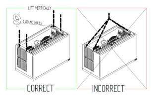
For the lifting and transport of the rest of the models, suitable equipment or machinery must be used for this purpose, such as pallet trucks, forklifts, etc., to ensure the lifting of the machine without causing any damage to the equipment or personnel carrying out the operation. The equipment must be properly packed and protected to avoid cosmetic or mechanical damage during transport.
