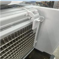
**4-.** Replace the tray, first one left coupling and then the other. Check for proper operation.
