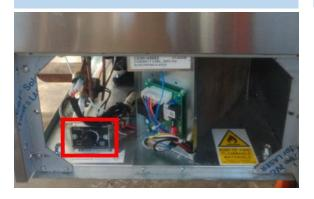
**2-.** The thermostats can be adjusted from position 1 (highest temperature 11°C) to position 7 (lowest temperature 4°C).
