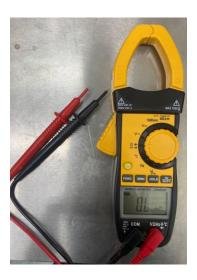
**2-.** Place the tester in the correct position to measure ohms ( $\Omega$ ) and check that the probe gives a value of 10k at an ambient temperature of 25°C. If the result is less than 10K, replace the probe.
